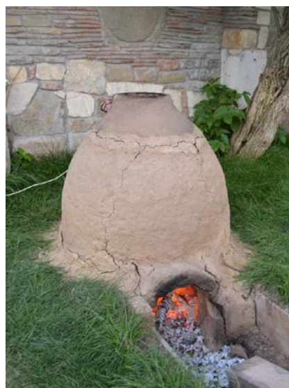
Figure 6. The kiln during firing (640°C).
