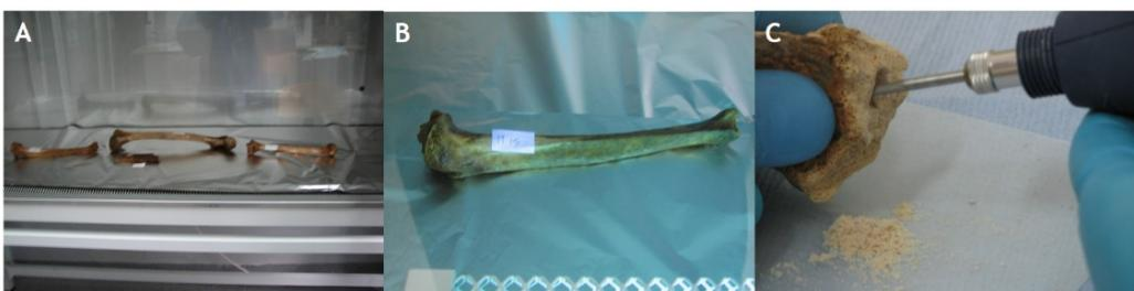
Figure 4. Samples preparation steps: (A) drying after sodium hypochlorite wash, (B) UV exposure, and (C) bone powder sampling.
