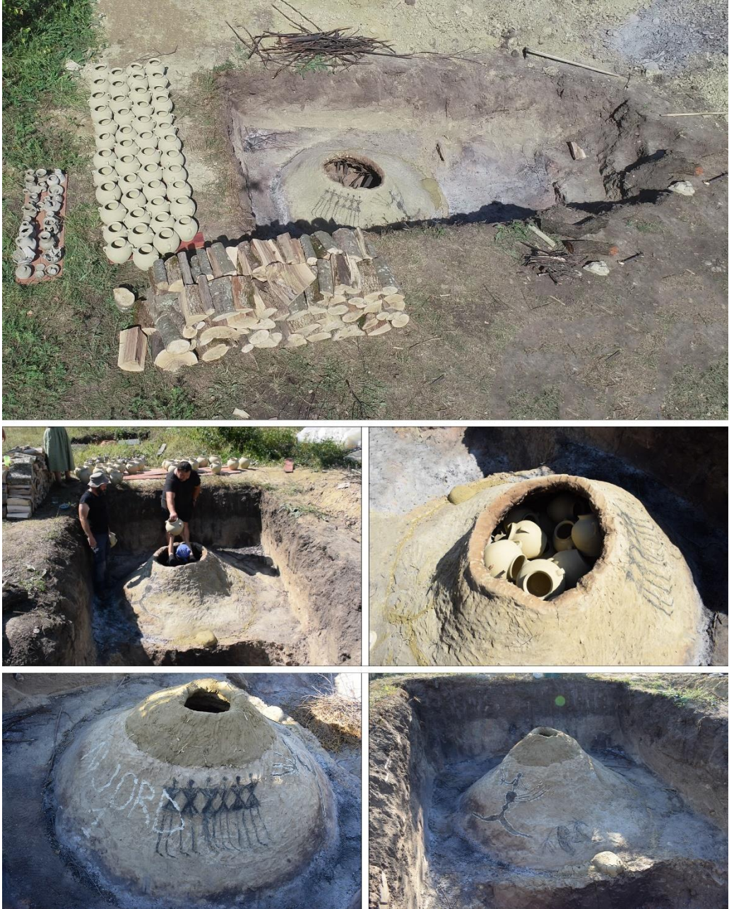
Fig.4. The experimental kiln after the initial drying
