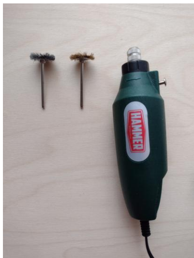
Figure 2. A tool for cleaning coins from solid deposits (Hammer MD 050 B mini drills with nozzles). (photo by the authors).
